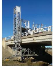
This lightweight truck has a 7 metre platform which makes it ideal for bridges with a low weight limit which require a maximum amount of reach. The platform is capable of being deployed in such a way that it can act as a temporary guard rail if needed and the units size combined with its smaller profile makes it perfectly suited for working on narrow bridges or bridges where the pylons are close together.
