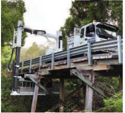
Lightweight and super mobile this unit is ideal for bridges with a low weight limit or hard to reach areas. It is capable of deploying from left, right and rear of the truck making it perfect for use on jetties or wharfs.
