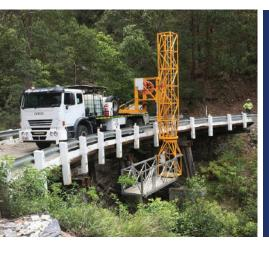
This is the beast of our fleet. Its a 7m Moog platform mounted on a dual control Acco with permanently fixed generator, screw compressor, pressure cleaner and water tank.
