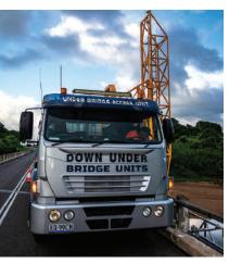
This platform is fitted with dual controls and a sidewalk extension, making it easier to navigate tighter bridges. Combine this with the capability to extend 9m horizontally along edge of bridge, makes for an extremely versatile machine.
