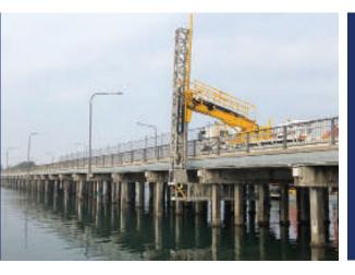
The 7 – 13 metre Barin Industrial platform has the capacity to reach out 4m while launching over a 3.8m barrier. It has an 11 metre platform capable of being loaded with 500kg of personnel and equipment and comes fully loaded with a generator, screw compressor, gurney and the ability to carry 1000L of water. All this capacity makes its it the perfect work horse to support any major project
