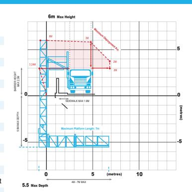
This is another of our lightweight machines. Its got a 7m platform which can handle 400kg work load evenly spread across it.
