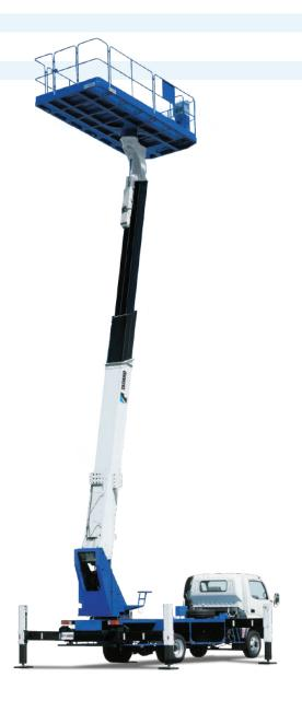
This is one of the newest acquisitions to our fleet. It deploys up rather than down however its huge platform, capable of being deployed 19.7m into the air has a safe working load of 1000kg.
