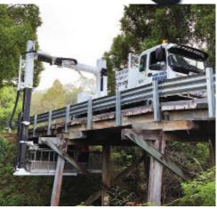
Lightweight and super mobile this unit is ideal for bridges with a low weight limit or hard to reach areas. It is capable of deploying from left, right and rear of the truck making it perfect for use on jetties or wharfs.
