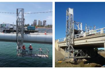
This lightweight truck has a 7 metre platform which makes it ideal for bridges with a low weight limit which require a maximum amount of reach. The platform is capable of being deployed in such a way that it can act as a temporary guard rail if needed and the units size combined with its smaller profile makes it perfectly suited for working on narrow bridges or bridges where the pylons are close together.
