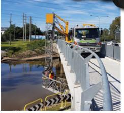
This is another of our lightweight machines. Its got a 7m platform which can handle 400kg work load evenly spread across it.
