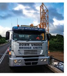
This platform is fitted with dual controls and a sidewalk extension, making it easier to navigate tighter bridges. Combine this with the capability to extend 9m horizontally along edge of bridge, makes for an extremely versatile machine.
